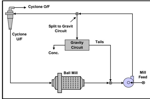
Figure 4. Typical grinding circuit incorporating gravity concentration
