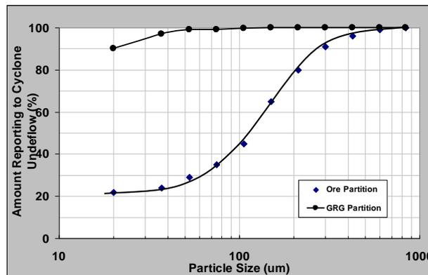
Figure 3. Typical partition curves for ore and GRG
