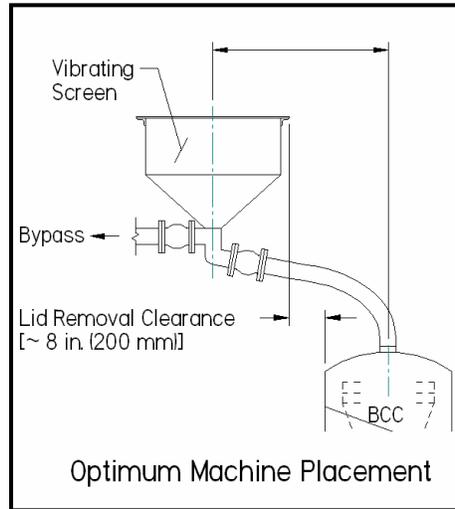
**Figure 7. BCC placement relative to sizing screen.**
