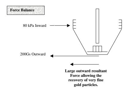
Falcon prides itself in the recovery of very fine gold particles (below 10 microns), this can only be achieved with the use of low water pressures to fluidize the concentrate riffles (50-80 kPa) and with high outward G-forces (200Gs). Other equipment encountered in the industry make use of high water pressures and lower G-forces resulting in the ejection of fine gold from the collected concentrate.
